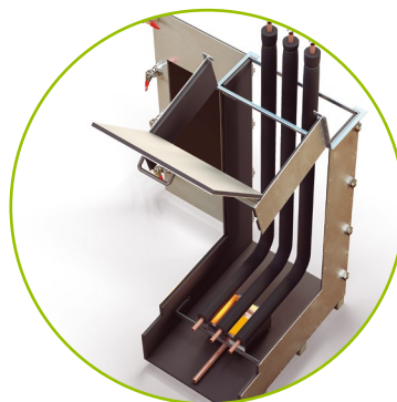
A small, growing fire which escalates is placed directly underneath the pipes and the fire performance is observed.
